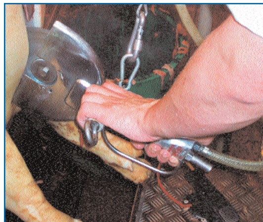
Jarvis' Model SPC 165B Circular Brisket Saw cuts hog briskets quickly and accurately.
