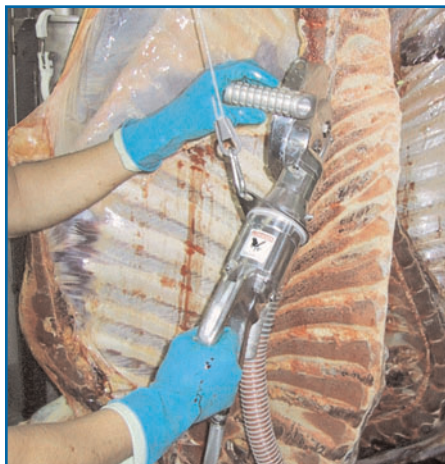
Photo of a Jarvis saw effectively removing spinal cord material from a beef carcass.
