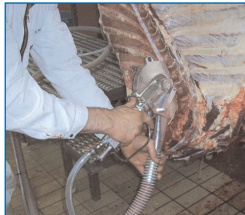
The SPC 165G provides a cost-effective and highly efficient method for better and faster spinal cord removals.
